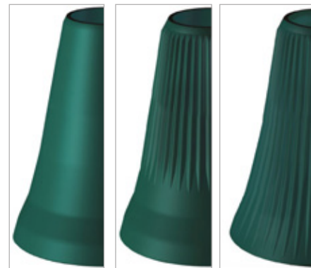
Examples of smooth (left), partially corrugated (center) and fully corrugated (right) mantle profiles.
